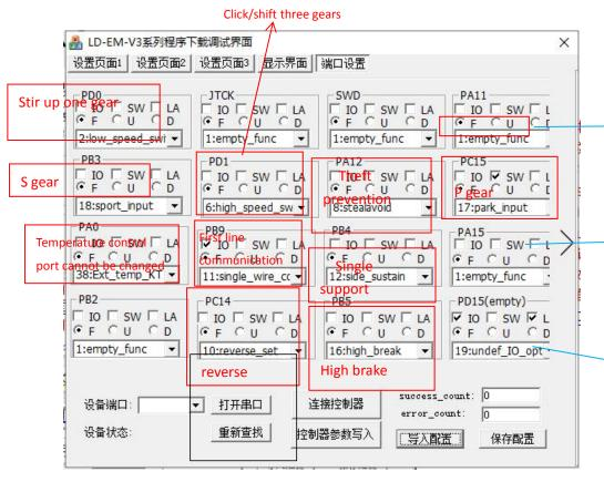
6.1: the above port functions are factory default configuration, corresponding to Lande 2×8 transfer line drawing, em30s EM50 (EM100 without anti-theft) -EM150s is general.
