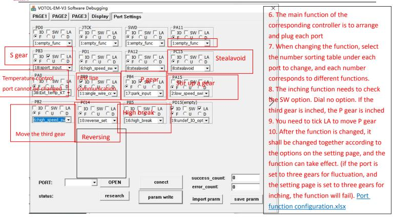
6.2: the above port functions are factory default configuration, corresponding to Lande  $2 \times 8$  transfer line drawing, and EM100 is dedicated with anti-theft harness.
