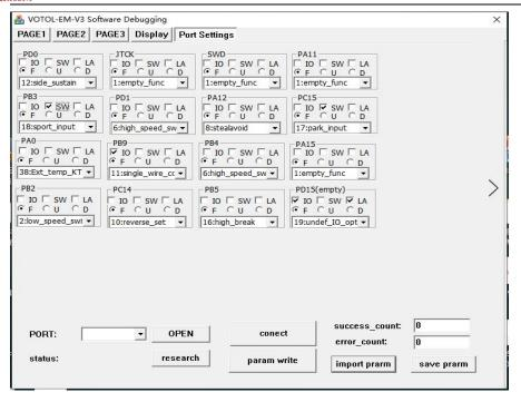
6.3: the above port functions are factory default configuration, corresponding to Lande  $2 \times 8$  transfer line drawing, dedicated to em150sp (after 20200321) controller.
